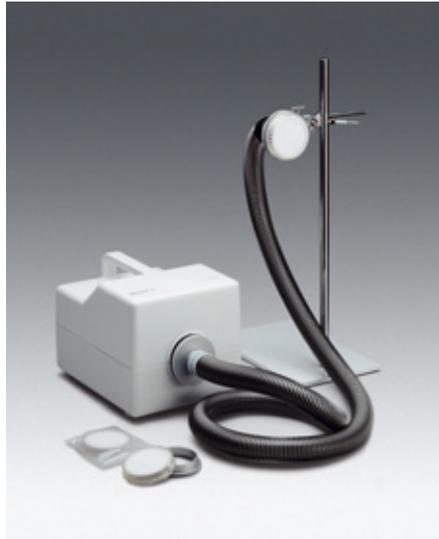
MD8 airscan Air Sampler with Gelatin Filter Disposable
